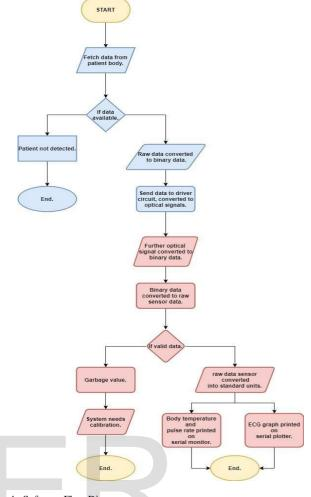
Fig. 4. Software Flow Diagram
