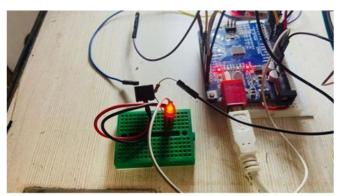
Fig. 8. LED & Buzzer "ON" State indicating Emergency at Patients' Unit
