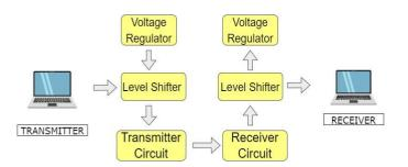
Fig. 2. Working Principle of Li-Fi Technology [3]
